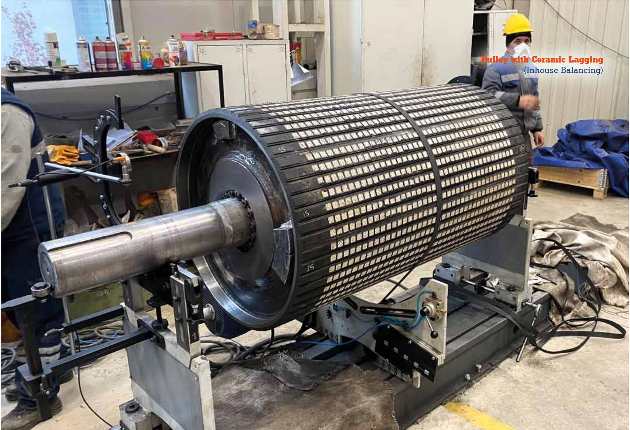
**Pulley with Ceramic Lagging**
